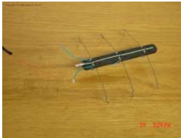
Figure 1: A basic walking Stiquito™ robot.
